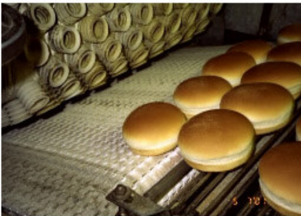
uni Light CR moving buns up an incline
