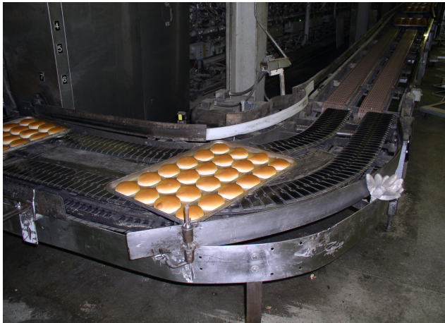
The picture above shows a traditional system using 2 lanes of steel chain. Today this will be made with uni Flex SNB with SS reinforcing links.
