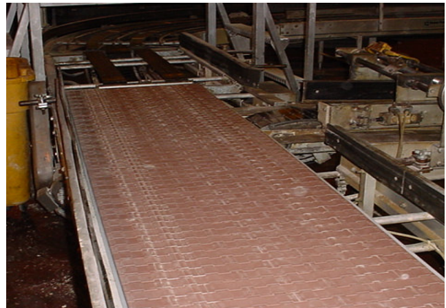
The same conveyor fitted with single lane uni SSB closed in LF material
