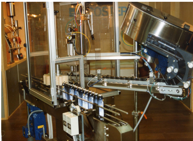
uni 820 chain on a capper machine
