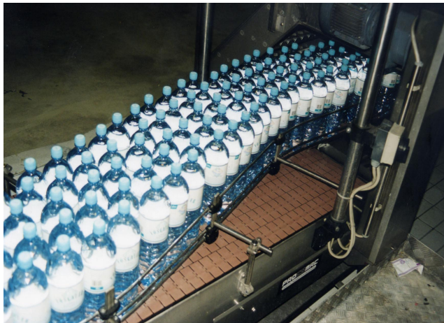
uni 820 chain moving plastic bottles
