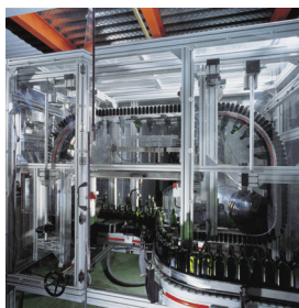
uni 1873 chain with G4 grippers in various gripper elevator applications
