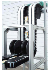
uni 1873 chain with G4 grippers in various gripper elevator applications
