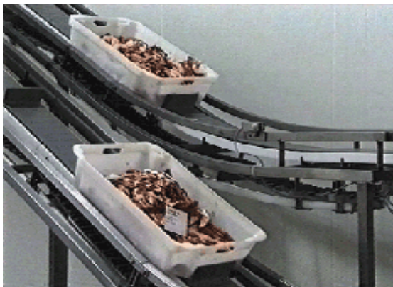
Uni SNB M2 20% Rubber Top conveying totes
