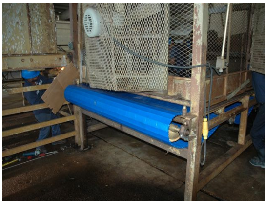
uni MPB in PEI blue material on a cage dump conveyor
