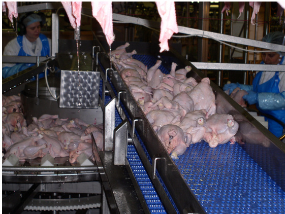
uni MPB 22% open on a chiller discharge conveyor
