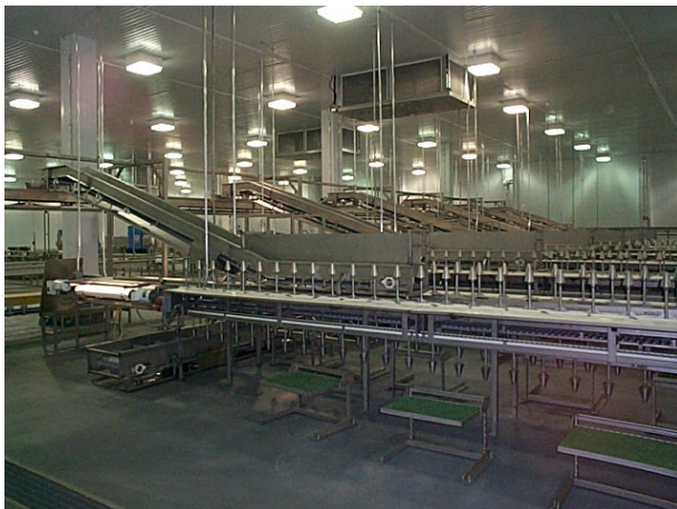
uni 3200 TAB chain on a cone line (moving deboning line)
