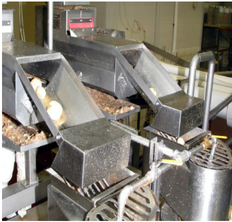
Peeled potatoes slide onto a uni MPB closed in PP material with PA6.6 pins below.
