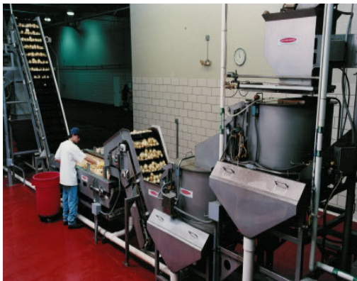
uni MPB in PP material with PA6.6 pins and Product Supports for a Incline Conveyor to the Peeler.
