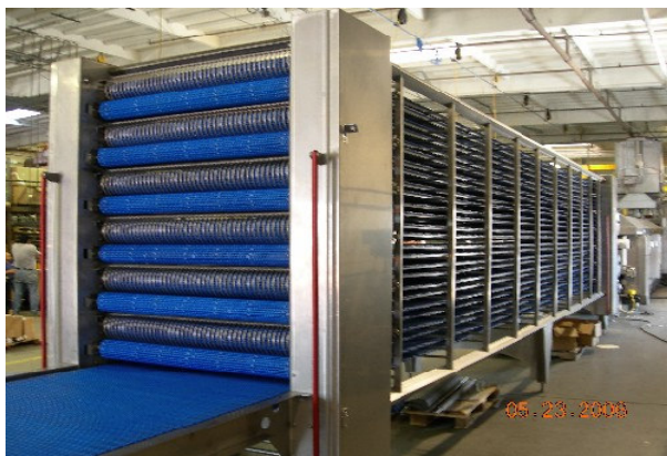
Above a multi-tier tortilla cooler using uni SNB M2 34% open in PA6.6 (nylon)
