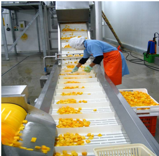
uni Light EP 18% on a mango incline conveyor
