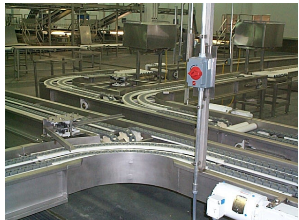
uni 3200 TAB chain on some dual lane crate conveyors
